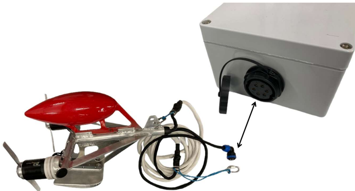
Figure 11: Hydrogenerator directly connected to the electrical box
